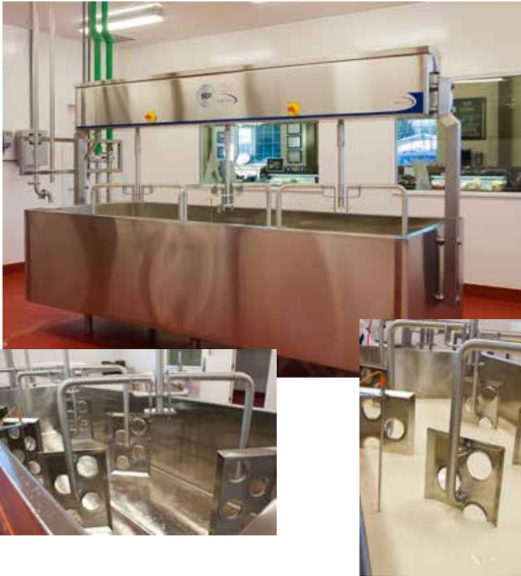
The Horizontal Open Vat is designed to agitate end to end in a pattern that assures no laminar flow, something that can't be achieved in a round vat. The agitation pattern assures even heat distribution transfer.
